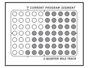
the first segment is shown in the flashing CUR-RENT SEGMENT column of the LED matrix. (The incline settings are not shown in the matrix.) The settings of the next seven segments are shown in the columns to the right.
